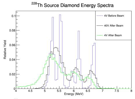
**Fig. 2**.  $^{228}$ Th alpha spectra in Diamond-DADL telescope configuration. Black is the  $^{228}$ Th spectra with the diamond biased to +40 V while in green it is biased at +4 V. In blue is the same detector biased at +4 V before the experiment.
